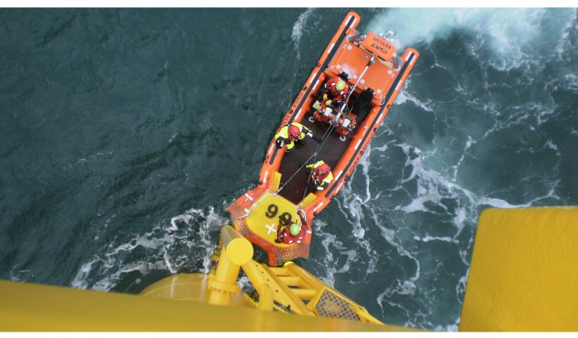
ESVAGT has modified the stern of the FRB 15 C, so that they are specially suited to dock at the offshore wind platforms.
