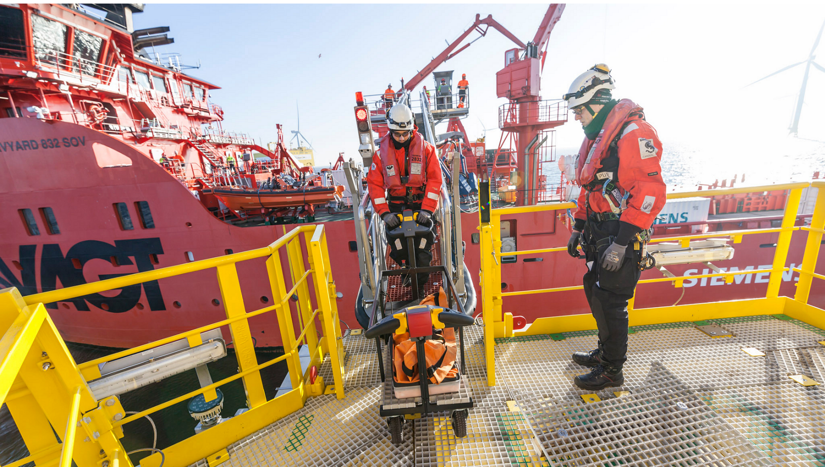
Transfer of specialists, tools and parts from 'Esvagt Froude' to a wind turbine by Ampelmann walk to work gangway.
