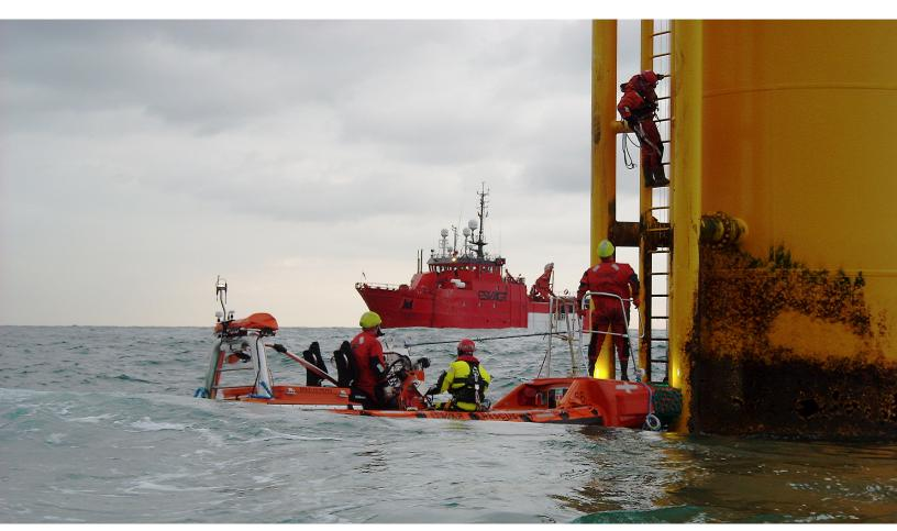
The contract between MHI Vestas Offshore Wind and ESVAGT reiterates that ESVAGT's concept of using Safe Transfer Boats to transfer technicians and spare parts safely from vessel to turbine is a success.
