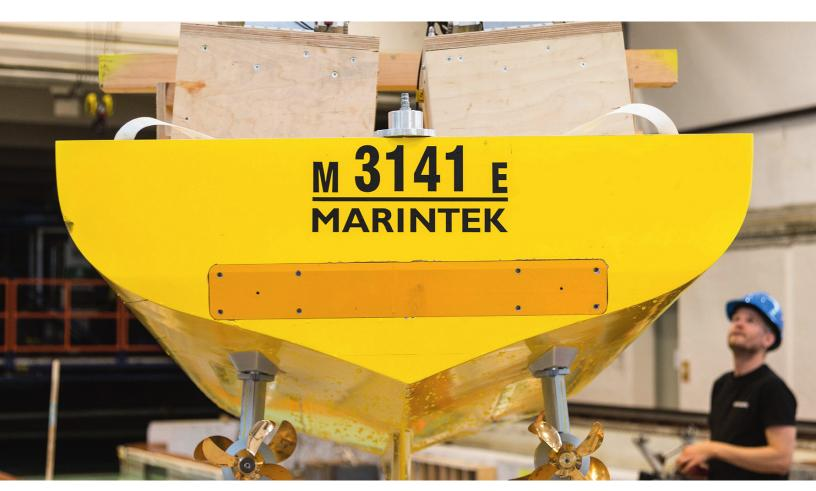
The hull of the new vessel has been through about 100 calculations. The same level of detail has influenced the propulsion system and propellers, which have also been thoroughly tested to ensure optimal performance at 15 knots.
