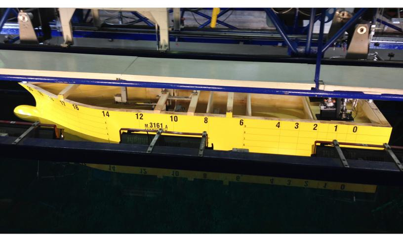
The model tests of the SOV for MHI Vestas demonstrates excellent hull drag
