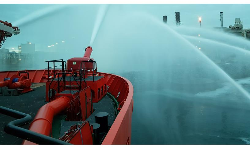
The 'Esvagt Aurora' is equipped with two state-of-the-art and powerful Fi-Fi cannons (fifi = fire fighting, red.), which are able to "shoot"  $2 \times 60,000$  litres of water per minute at a distance of 180 metres and a height of 110 metres.
