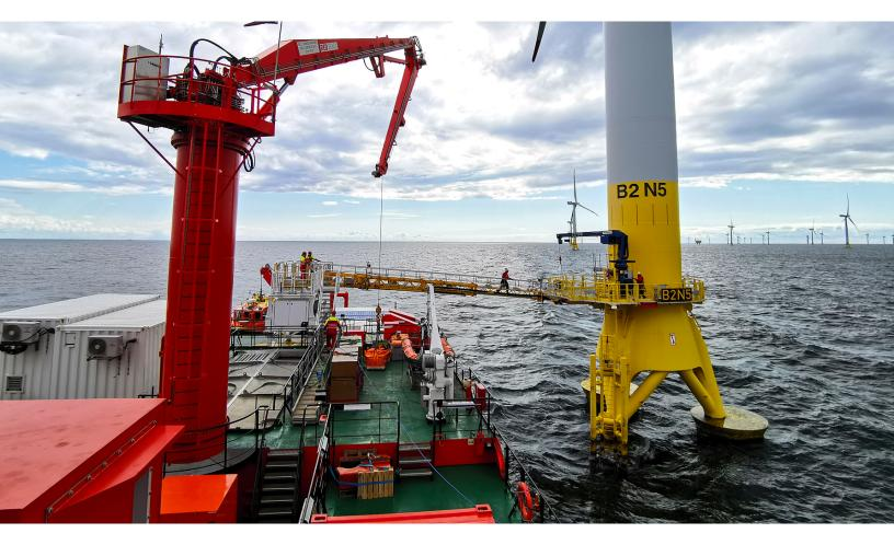
The 'Esvagt Dana's gangway can operate to both sides and safely transfer technicians to the offshore wind turbine.
