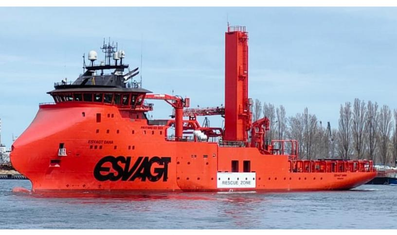
The weather in the North Sea required a modification of 'Esvagt Dana and the vessel has become four meters wider. At the same time, the gangway system has been re-designed so that it is stepless and can access the different heights on the North Sea's
