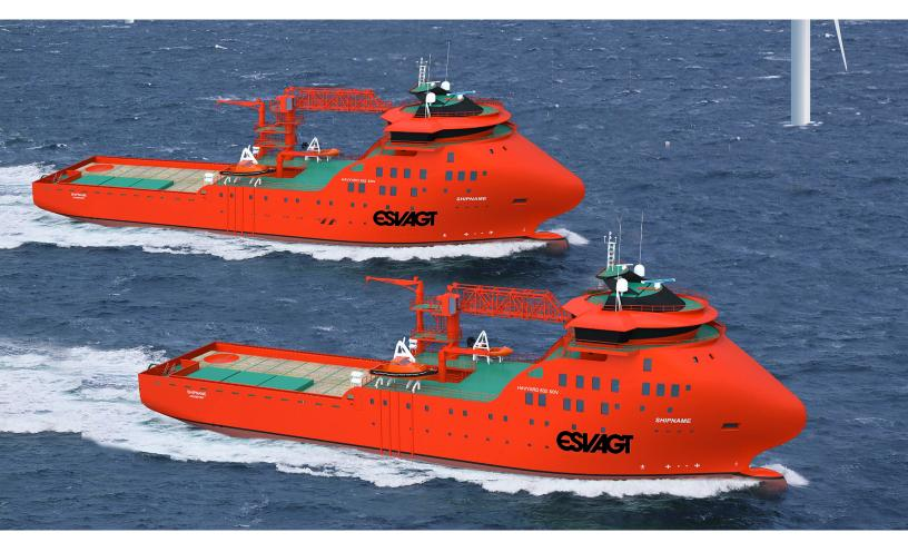
The purpose-built SOVs will be equipped with Walk-to-work gangways that can be used to transfer technicians to the platforms 22 metres above the surface of the sea. The gangway is stabilized so that it can land people in waves even 2.5-metre high.
